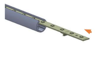
**Step 1**Cabling LED-Strips and slide into the profile.
