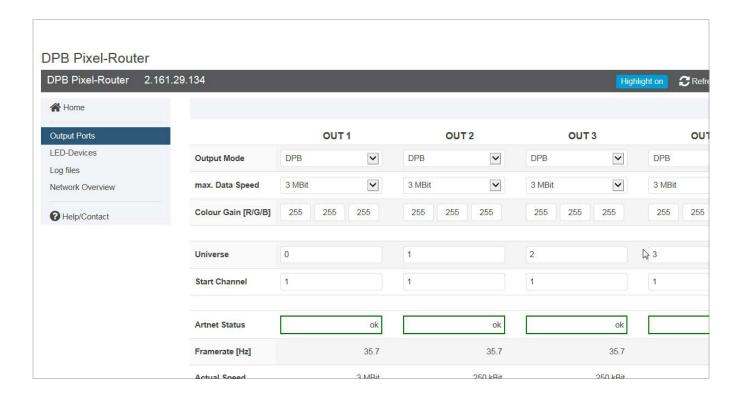
Under the menu item "Output Ports", you can find the overview of the device outputs. This is where you can set the Output Mode, the maximum Data Speed of the Colour Gain and the Combine Mode.
