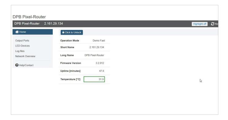
This is where the DPB Pixel-Router's basic data is displayed.
